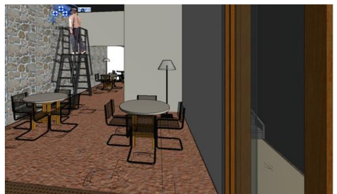
Figure 6 - Placement of the ladder for servicing of the air conditioning equipment
